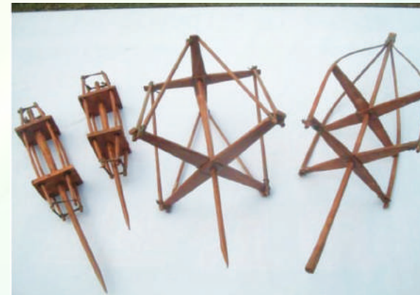
Small winder and big winder of yarn in Assam
